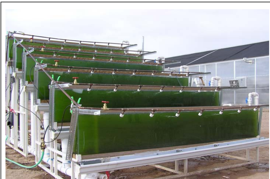
Figure 12. Operation of the multi-stage, continuous-flow photobioreactor for groundwater nitrate removal by Scenedesmus cells.
