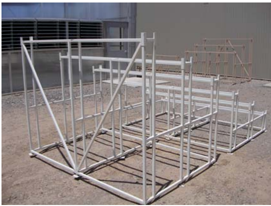
Figure 2. A welded steel frame made of 1" square tubing for bioreactor support.
